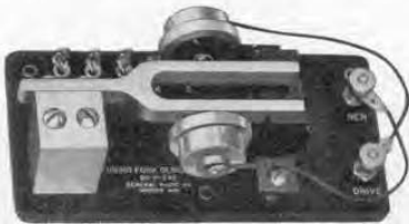
FIGURE 5. A double-button microphone-driven fork. Note the heavy brass inertia caps which house the microphone buttons
